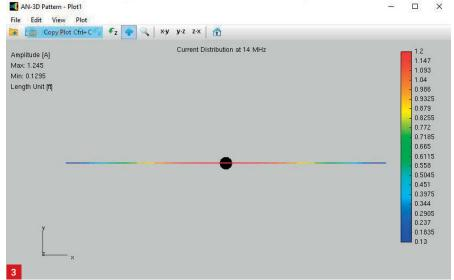
Fig. 1: Electromagnetic Waves. Fig. 2: A diagram of  $\lambda/2$  dipole elements (top), with current and voltage plots below. Fig. 3: An AN-SOF simulation of currents along a 20m dipole element. Fig. 4a: An AN-SOF simulation of a horizontal 20m dipole in free space. Fig. 4b: An AN-SOF simulation of a vertical dipole in free space. Fig. 5: An AN-SOF simulation of a 20m dipole  $\lambda/2$  above ground. Fig. 6: An AN-SOF simulation of the same 20m dipole but at 4 $\lambda$  above ground.
