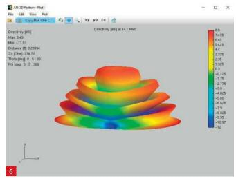
of a 14MHz horizontal dipole at  $\lambda/2$  (33ft) above a *realistic* ground. It can be seen that ground greatly affects the radiation pattern. This pattern is also affected by what ground type is below the aerial. Built-up areas are generally quite poor, while seawater on the other hand is excellent in this respect.
